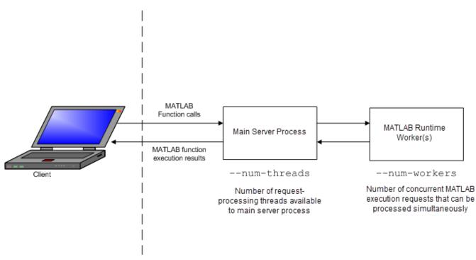
• Threads (throughput management) (num-threads) — The number of threads (units of processing) available to the main server process.
